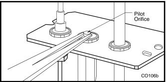
Fig. 62 Remove pilot orifice.
